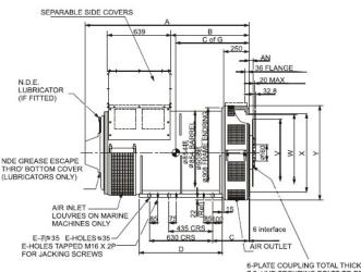
6-PLATE COUPLING TOTAL THICKNESS 7,2. HUB SECURING BOLTS TO BE TIGHTENED TO A TORQUE OF 84kgfm 822Nm
